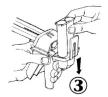
Drop in the syringe. Return the holder to original position and snap catch back into place. Dispense product by squeezing trigger.
