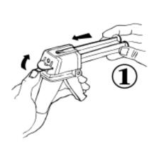
Insert plunger, track side down, into slot on front face of the applicator. Push up the metal lever on the back of the applicator and slide the plunger full length into the applicator.
