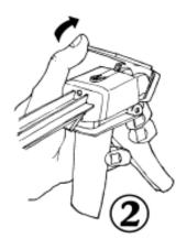
Lift up the plastic catch on the syringe holder bracket.
